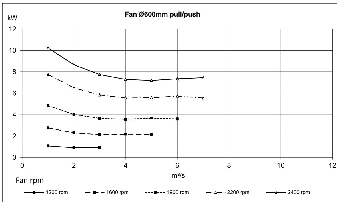
Maximum fan speed with visco clutch: 2400rpm
