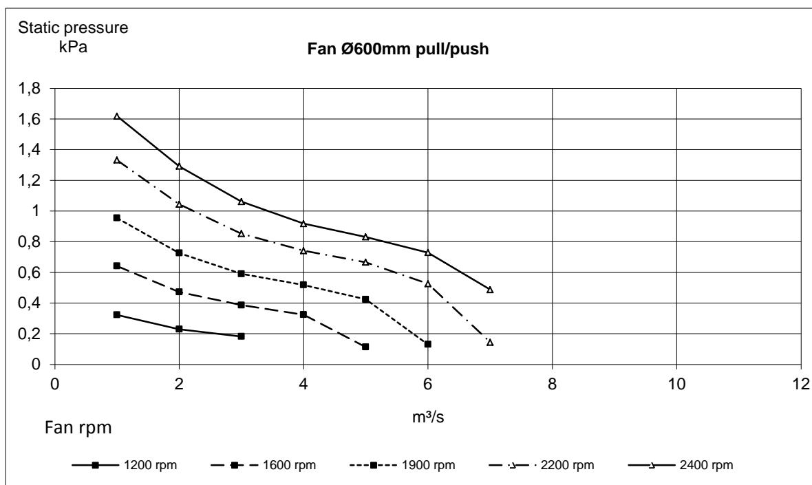
Maximum fan speed with visco clutch: 2400rpm
